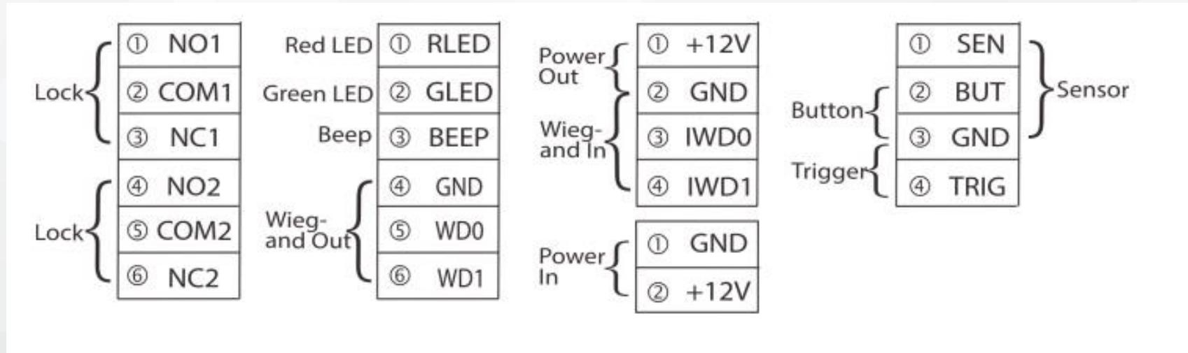
2 relay output, wiegand out, wiegand in, door magnetic, door exit trigger ( One relay is for lock , two relay is for alarm)
